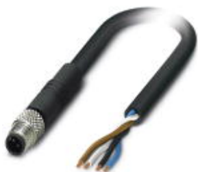
Sensor/Actuator cable, 4-position, PUR, black RAL 9005, Plug straight M5, A-coded, on free cable end, Cable length: 5 m
