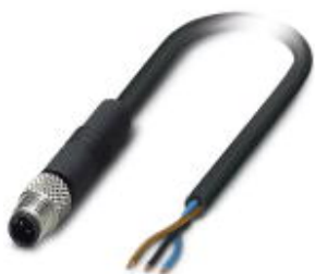
Sensor/Actuator cable, 3-position, PUR, black RAL 9005, Plug straight M5, A-coded, on free cable end, Cable length: 3 m
