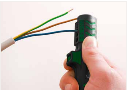
Stripping a wire insulation.
