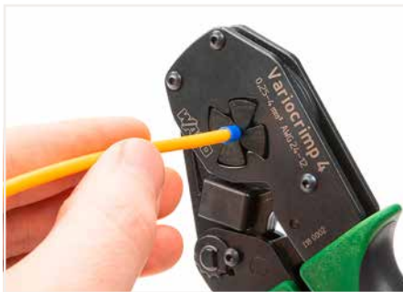
Squeeze handles until ratchet mechanism is released.
