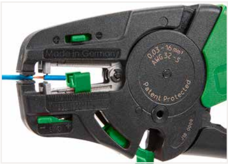
Partially stripping a conductor.
