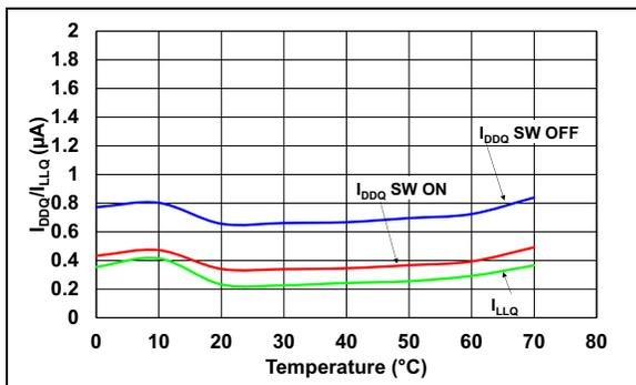
FIGURE 4-3:  $I_{DDQ}/I_{LLQ}$  vs. Temperature.
