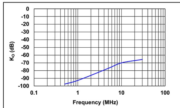
FIGURE 4-6:  $K_O$  vs. Frequency with 50Ω Load.
