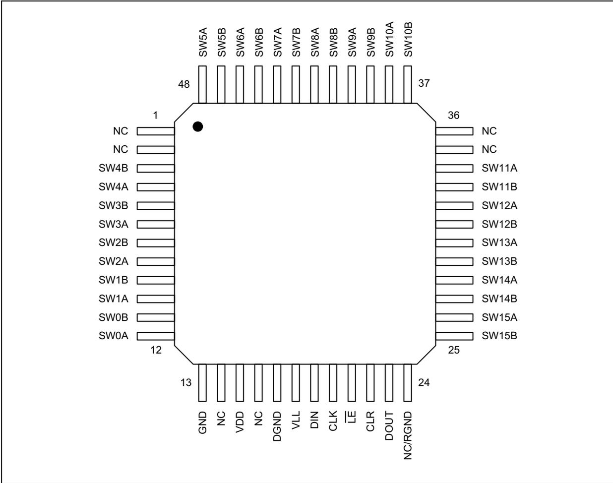
**FIGURE 2-1:** 48-Lead LQFP Package – Top View.
