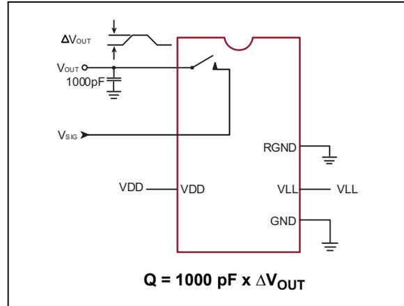
**FIGURE 3-9:** Charge Injection.
