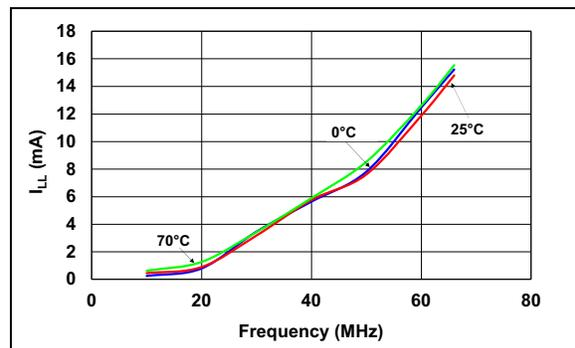
FIGURE 4-5:  $I_{LL}$  vs. CLK Frequency.
