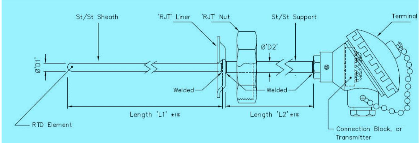
RJT unions (Ring Joint Type) are often referred to as a standard union. The compromise of an O-ring style gasket which leaves a small crevice where the liner and male part of the union overlap.
