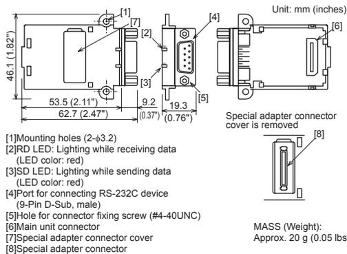
The communication port of the FX3U-232-BD is a 9-Pin D-Sub male type. The table below shows the pin arrangement.
