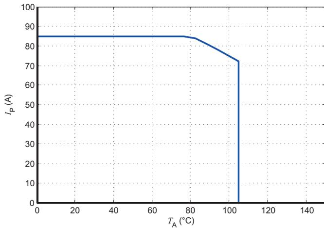
Figure 23:  $I_p$  vs  $T_A$  for LKSR 25-NP
