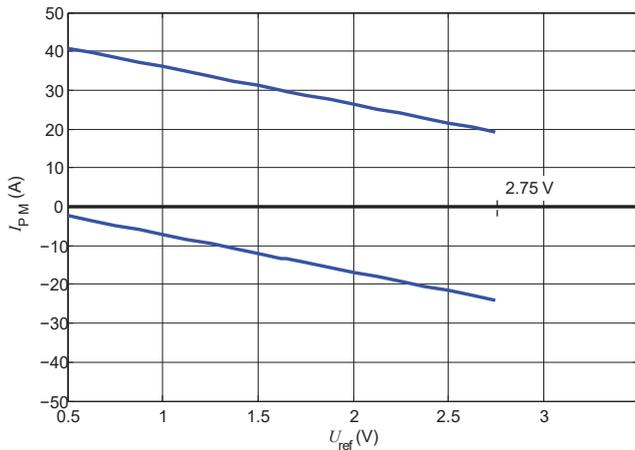
Figure 30: Measuring range versus external  $U_{ref}$  LKSR 6 A
