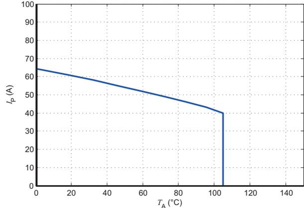
Figure 22:  $I_p$  vs  $T_A$  for LKSR 15-NP
