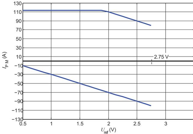
Figure 32: Measuring range versus external  $U_{ref}$  LKSR 25 A
