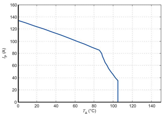
Figure 24:  $I_p$  vs  $T_A$  for LKSR 50-NP
