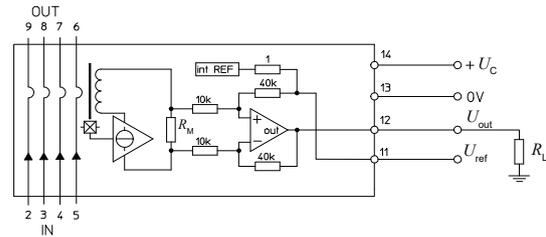
Figure 26: Test connection
