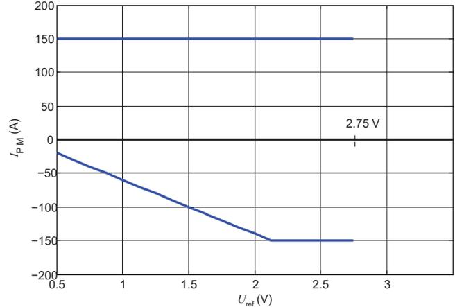
Figure 33: Measuring range versus external  $U_{ref}$  LKSR 50 A
