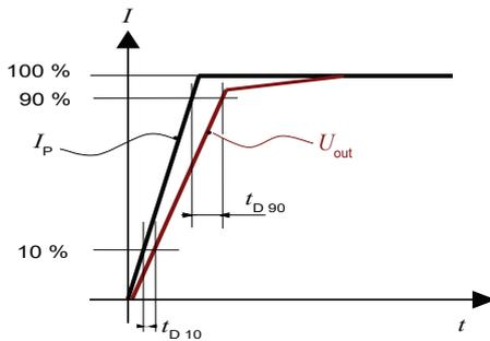
Figure 28:  $t_{D10}$  (delay time @ 10 %) and  $t_{D90}$  (delay time @ 90 %)
