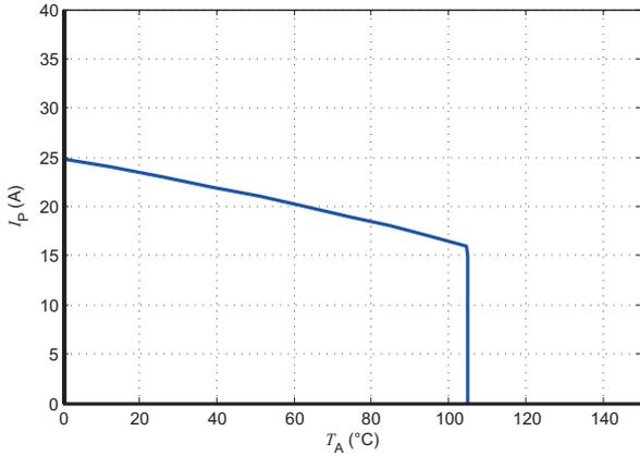
Figure 21:  $I_p$  vs  $T_A$  for LKSR 6-NP
