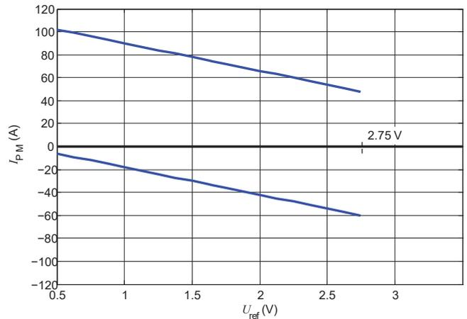
Figure 31: Measuring range versus external  $U_{ref}$  LKSR 15 A
