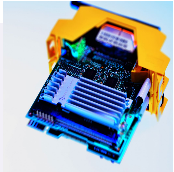
Brainboxes BB-400 with custom aluminium heatsink
