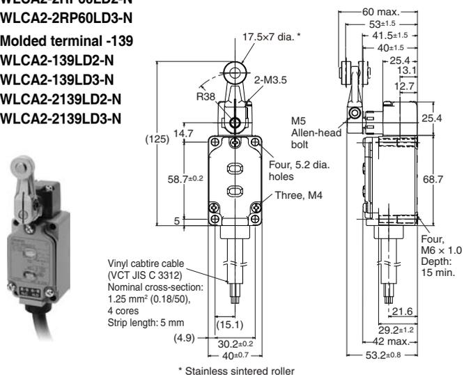
Note: The photo shows the WLCA2-RP60LD3-N model.
