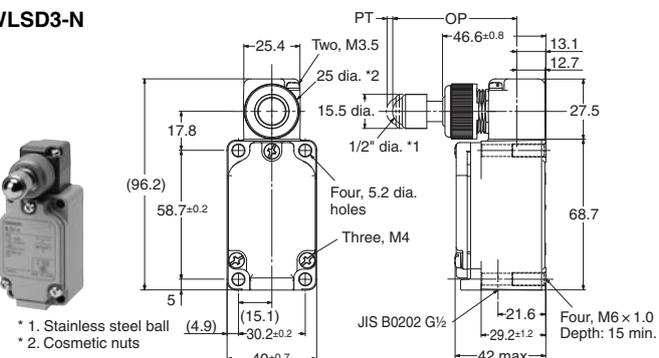
Horizontal-ball plunger With operation indicator
