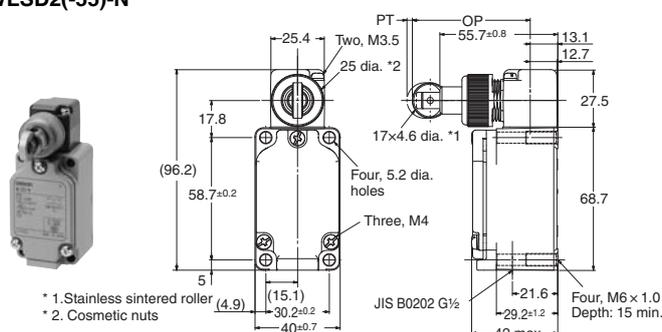
Horizontal-roller plunger With operation indicator
