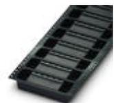
Header, nominal current: 12 A, rated voltage (III/2): 320 V, number of positions: 8, pitch: 5.08 mm, Color: black, contact surface: Tin, mounting: THR soldering, User information and design recommendations for through hole reflow technology can be found under "Downloads"
