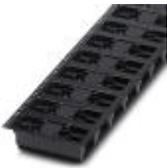
Header, nominal current: 12 A, rated voltage (III/2): 320 V, number of positions: 8, pitch: 5.08 mm, Color: black, contact surface: Tin, mounting: THR soldering, User information and design recommendations for through hole reflow technology can be found under "Downloads"
