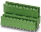
Header, nominal current: 10 A, rated voltage (III/2): 320 V, number of positions: 8, pitch: 5.08 mm, Color: green, contact surface: Tin, mounting: Wave soldering, Can be aligned! Mounting flange: Order No. 1836477, 1836480. In combination with MVSTB or FKCV plug components, both an MVSTBW (or FKCVW) and an MVSTBR plug (or FKCVR) must be used. Combination with TMSTBP plug components is not possible!
