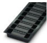
Header, nominal current: 12 A, rated voltage (III/2): 320 V, number of positions: 5, pitch: 5.08 mm, Color: black, contact surface: Tin, mounting: THR soldering, User information and design recommendations for through hole reflow technology can be found under "Downloads"
