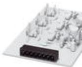
Header, nominal current: 12 A, rated voltage (III/2): 320 V, number of positions: 5, pitch: 5.08 mm, Color: black, contact surface: Tin, mounting: THR soldering, User information and design recommendations for through hole reflow technology can be found under "Downloads"
