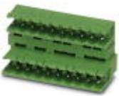
Header, Nominal current: 10 A, Rated voltage (III/2): 320 V, Number of positions: 8, Pitch: 5 mm, Color: green, Contact surface: Tin, Mounting: Wave soldering, Can be aligned! Mounting flange: Order No. 1736771, 1736768. In combination with MVSTB or FKCV plug components, both an MVSTBW (or FKCVW) and an MVSTBR plug (or FKCVR) must be used. Combination with TMSTBP plug components is not possible!
