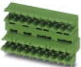
Header, Nominal current: 10 A, Rated voltage (III/2): 320 V, Number of positions: 8, Pitch: 5 mm, Color: green, Contact surface: Tin, Mounting: Wave soldering, The article can be aligned to create different nos. of positions! In combination with MVSTB or FKCV plug components, both an MVSTBW (or FKCVW) and an MVSTBR plug (or FKCVR) must be used. Combination with TMSTBP plug components is not possible!
