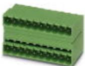
Header, Nominal current: 10 A, Rated voltage (III/2): 320 V, Number of positions: 8, Pitch: 5 mm, Color: green, Contact surface: Tin, Mounting: Wave soldering, In combination with MVSTB or FKCV plug components, both an MVSTBW (or FKCVW) and an MVSTBR plug (or FKCVR) must be used. Combination with TMSTBP plug components is not possible!
