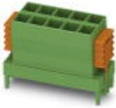
PCB direct plug, nominal current: 12 A, rated voltage (III/2): 320 V, nominal cross section: 2.5 mm<sup>2</sup>, number of positions: 4, pitch: 5 mm, connection method: Crimp connection, color: green, contact surface: Tin, mounting: SKEDD
