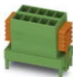
PCB direct plug, nominal current: 8 A, rated voltage (III/2): 160 V, nominal cross section: 1.5 mm<sup>2</sup>, number of positions: 3, pitch: 3.5 mm, connection method: Crimp connection, color: green, contact surface: Tin, mounting: SKEDD - Direct plug-in technology, pin layout: Linear pinning
