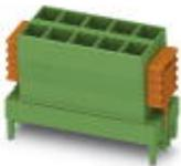
PCB direct plug, nominal current: 12 A, rated voltage (III/2): 320 V, nominal cross section: 2.5 mm<sup>2</sup>, number of positions: 6, pitch: 5 mm, connection method: Crimp connection, color: green, contact surface: Tin, mounting: SKEDD
