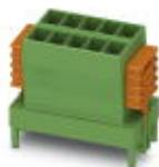
PCB direct plug, nominal current: 8 A, rated voltage (III/2): 160 V, nominal cross section: 1.5 mm<sup>2</sup>, number of positions: 2, pitch: 3.5 mm, connection method: Crimp connection, color: green, contact surface: Tin, mounting: SKEDD - Direct plug-in technology, pin layout: Linear pinning
