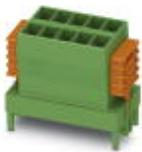
PCB direct plug, nominal current: 8 A, rated voltage (III/2): 160 V, nominal cross section: 1.5 mm<sup>2</sup>, number of positions: 5, pitch: 3.5 mm, connection method: Crimp connection, color: green, contact surface: Tin, mounting: SKEDD - Direct plug-in technology, pin layout: Linear pinning
