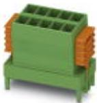
PCB direct plug, nominal current: 8 A, rated voltage (III/2): 160 V, nominal cross section: 1.5 mm<sup>2</sup>, number of positions: 7, pitch: 3.5 mm, connection method: Crimp connection, color: green, contact surface: Tin, mounting: SKEDD - Direct plug-in technology, pin layout: Linear pinning
