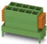
PCB direct plug, nominal current: 12 A, rated voltage (III/2): 320 V, nominal cross section: 2.5 mm<sup>2</sup>, number of positions: 5, pitch: 5 mm, connection method: Crimp connection, color: green, contact surface: Tin, mounting: SKEDD
