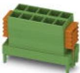
PCB direct plug, nominal current: 12 A, rated voltage (III/2): 320 V, nominal cross section: 2.5 mm<sup>2</sup>, number of positions: 7, pitch: 5 mm, connection method: Crimp connection, color: green, contact surface: Tin, mounting: SKEDD
