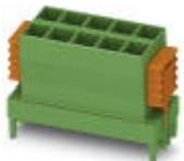
PCB direct plug, nominal current: 12 A, rated voltage (III/2): 320 V, nominal cross section: 2.5 mm<sup>2</sup>, number of positions: 2, pitch: 5 mm, connection method: Crimp connection, color: green, contact surface: Tin, mounting: SKEDD - Direct plug-in technology, pin layout: Linear pinning
