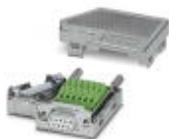
D-SUB connector, 9-pos. female connector, two cable entries < 35°, bus system: Modbus, Modbus Plus, BITBUS, ARCNET, MULT/MININET (B&R), SYSTEM 2003 (B&R), P-NET, pin assignment: 1, 2, 3, 5, 6, 8; screw connection terminal blocks
