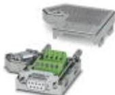
D-SUB plug, 9-pos. female connector, one cable entry < 35°, universal type for all systems, pin assignment: 1, 2, 3, 4, 5, 6, 7, 8, 9 to screw connection terminal block
