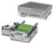
D-SUB connector, 9-pos. female connector, two cable entries < 35°, bus system: CAN, SUCONET K1, K2 (MOELLER), S-BUS (Saia), J-BUS (Merlin Gerin), pin assignment: 2, 3, 4, 5, 7, 9 to two screw connection terminal blocks
