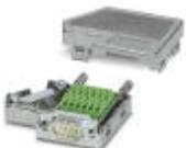
D-SUB connector, 9-pos., male connector, two cable entries < 35°, bus system: CAN, SUCONET K1, K2 (MOELLER), S-BUS (Saia), J-BUS (Merlin Gerin), pin assignment: 2, 3, 4, 5, 7, 9 to two screw connection terminal blocks
