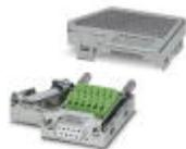
D-SUB connector, 9-pos. female connector, two cable entries < 35°, bus system: CAN, KEBA up to 1 Mbps, pin assignment: 2, 3, 4, 5, 6, 7; screw connection terminal blocks
