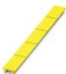
Contactor marker - zack marker strip, Strip, yellow, unlabeled, can be labeled with: CMS-P1-PLOTTER, mounting type: snap into flat marker groove, lettering field size: 20 mm x 8 mm, Number of individual labels: 5
