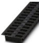
Header, nominal current: 8 A, rated voltage (III/2): 250 V, number of positions: 2, pitch: 3.5 mm, Color: black, contact surface: Tin, mounting: THR soldering. The maximum current depends on the plug used. The lower of the two current values apply for plug and pin strip. The pin strip is made of highly temperature resistant plastic and is thus suitable for the reflow process.
