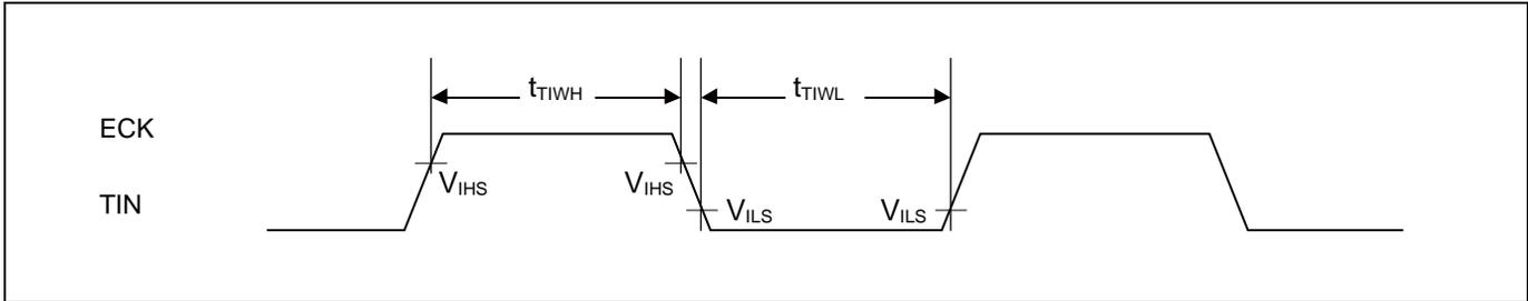
■ Trigger input timing
