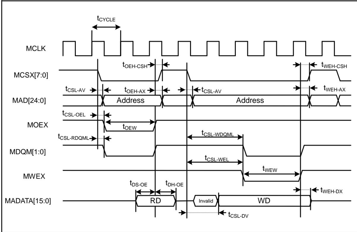
**■ Separate Bus Access Synchronous SRAM Mode**
