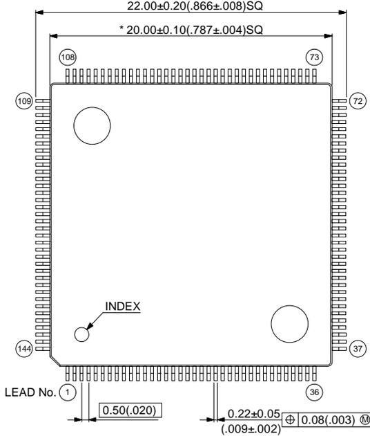
Note 1) \*:Values do not include resin protrusion.
