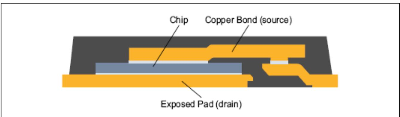
Figure 3 Cross section showing construction of a clip bond (e.g. TDSON)
