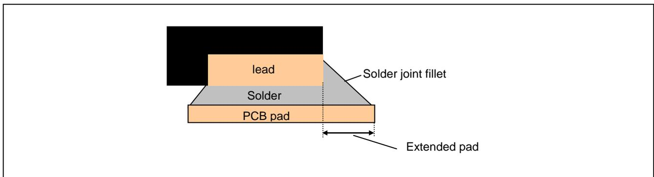
Figure 7 Schematic cross section of a perimeter lead
