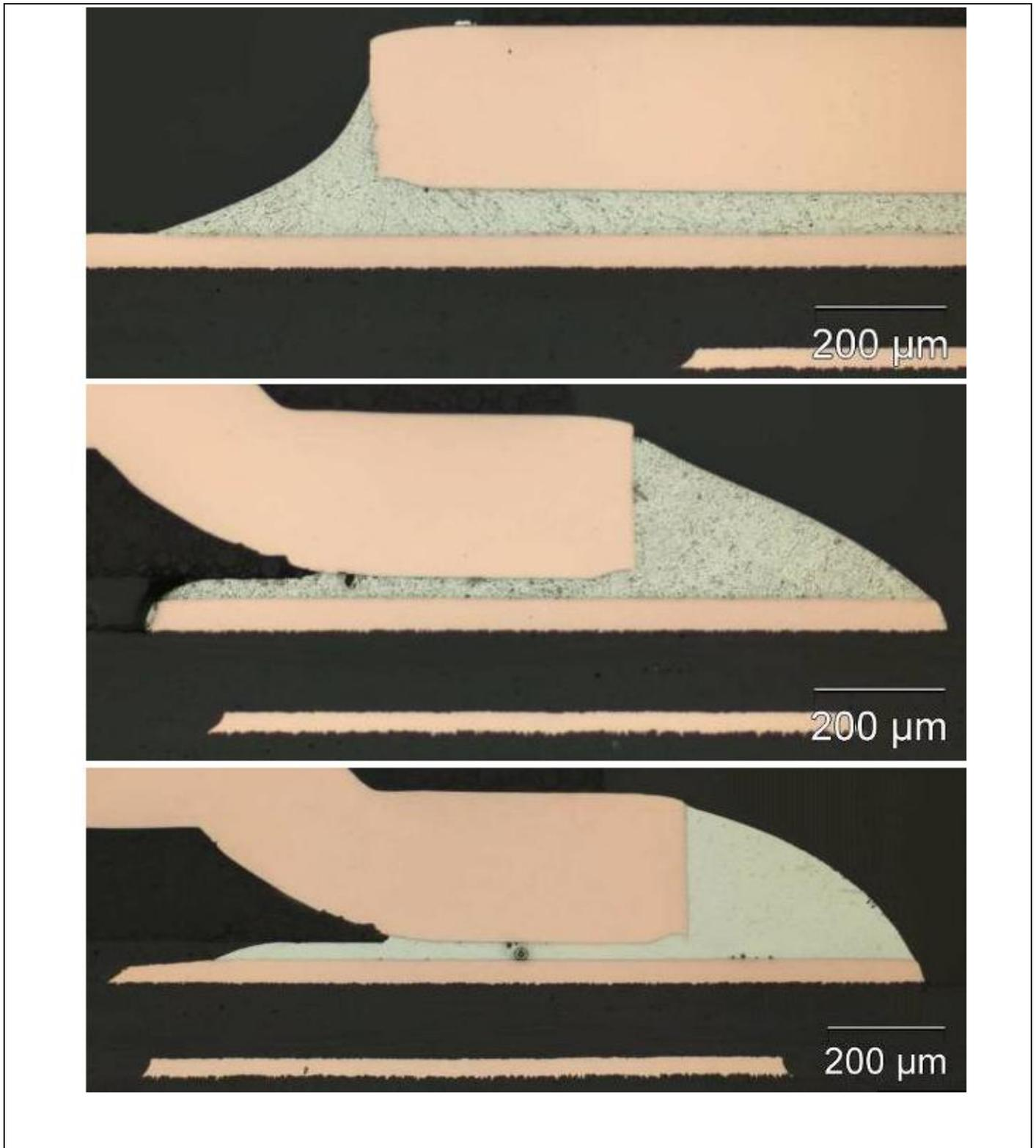
**Figure 14** Cross-section views of mounted TDSON-8 packages. The first photo shows a SnPb solder joint of the drain pad. The second and third photos show source/gate solder joints with SnPb, and SnAgCu alloys, respectively.
