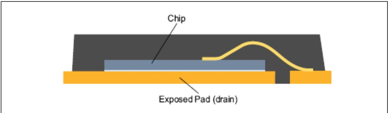
Figure 2 Cross section showing construction of a wire bond (e.g. TDSON)
