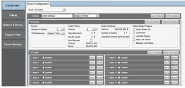
Use a USB to RS-485 adapter cable to connect a standalone DX80 Gateway to the computer. For DXM Controllers with an internal DX80 radio, connect a computer to the DXM Controller using a USB or Ethernet connection. Download the most recent revisions of the configuration software from Banner Engineering's website: [www.bannerengineering.com/wireless](http://www.bannerengineering.com/wireless).
