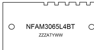
Device marking is on package top side
