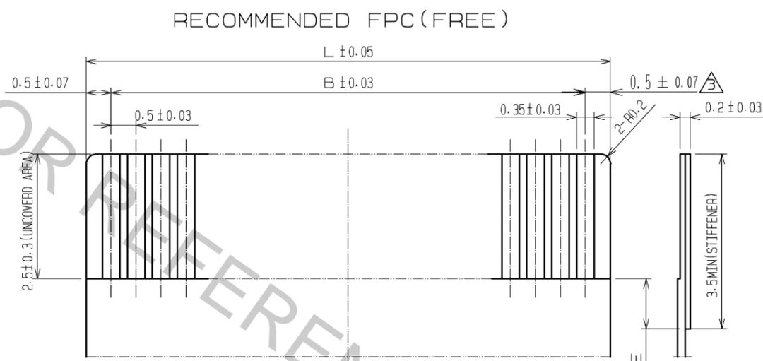
FOR FPC APPLICATION, STIFFENER MATERIAL IS POLYIMID, HEAT CURED ADHESIVE.
