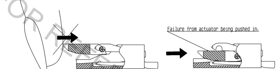
The actuator is designed to rotate on the axis shown in the figure below so make sure to use a rotating motion when operating it.
