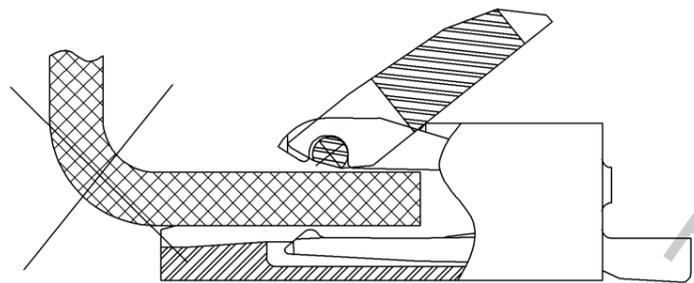
5. When inserting an FPC, do not use the method shown in the figure on the left below where the corner of the FPC is inserted first and then slid sideways. The FPC's corner can deform the terminal's contacts. Always insert the FPC parallel to the board as shown in the figure on the right below.
