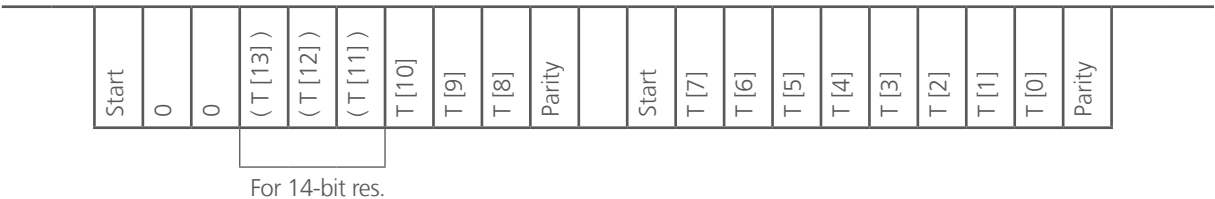
Figure 1.2 – Full ZACwire™ Temperature Transmission from TSic
