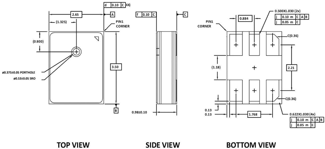
**Figure 16. 6-Terminal Chip Array Small Outline No-Lead Cavity**
