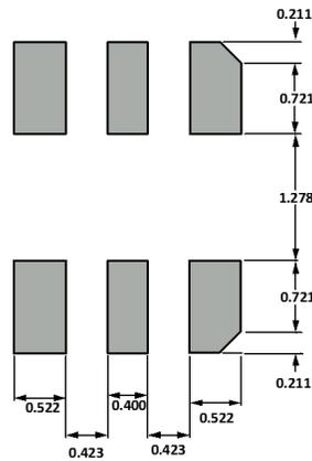
**Figure 15. Suggested Solder Paste Stencil Pattern Layout**
