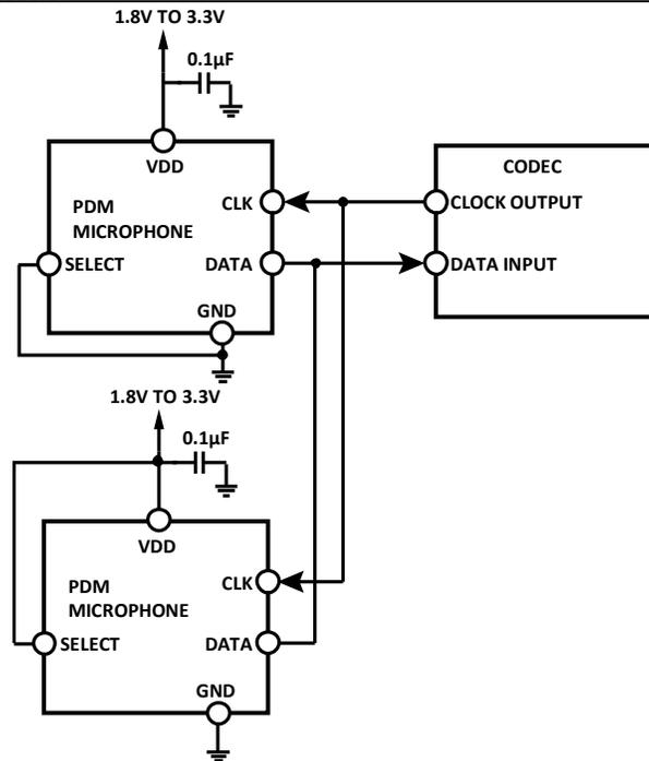
**Figure 12. Stereo PDM Microphone Connection to Codec**
