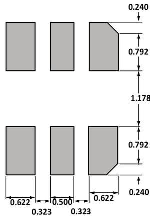
**Figure 14. Recommended PCB Land Pattern Layout**
