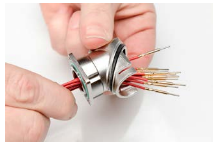
Step 4 - Crimp contacts onto wire
