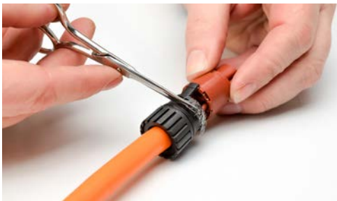
Step 14 - Trim shield as shown
