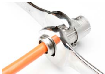
Step 17 - Tighten to 5-7 N/M using 25mm wrench
