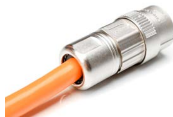
Step 17 - Tighten to 5-7 N/M using 25mm wrench
