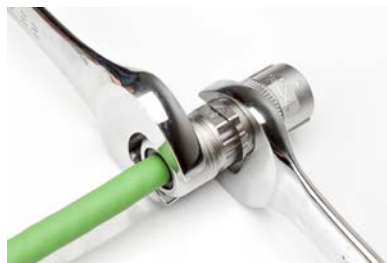
Step 16 - Tighten to 5-7 N/M using 25mm wrench
