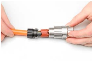
Step 15 - Push sub-assembly into shell
