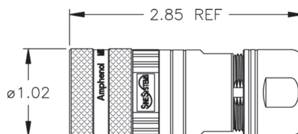
Plug kit straight, threaded; 7.5-11.0mm cord grip
