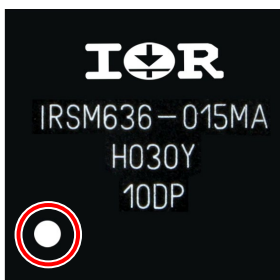
Figure 4 Pin 1 indicator on a \mu IPM PQFN device
