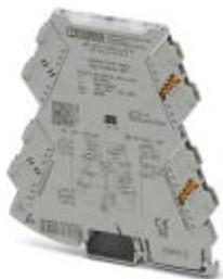
4-way power supply doubler with plug-in connection technology. HART-transparent, 0(4) mA ... 20 mA input signal, 0(4) mA ... 20 mA output signals. The device can be used in both signal and power supply doubler modes. Push-in connection technology.
