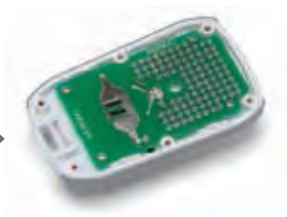
Install the PCB in the top cover
