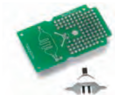
Solder the contacts onto the PCB
