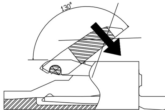
4. When operating the actuator, avoid operating it at its end. Make sure to operate it at its middle section.
