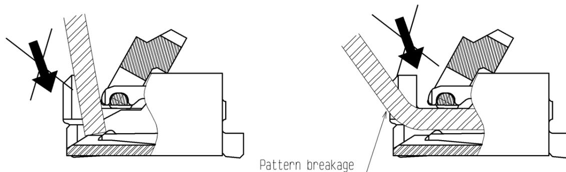
◆Checking the Locking Condition
