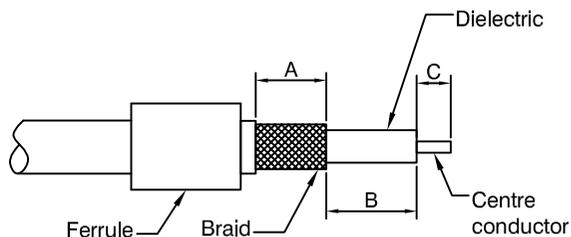
2) Position the contact on to the centre conductor and against the dielectric, crimp the contact using the toll indicated.
