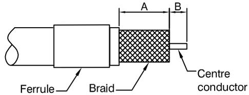
2) Crimp the contact onto the centre conductor.
