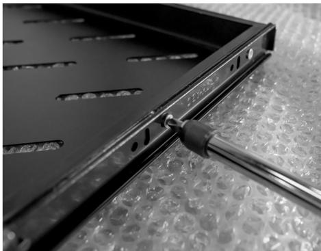
Locate and undo the three nuts on opposite side
