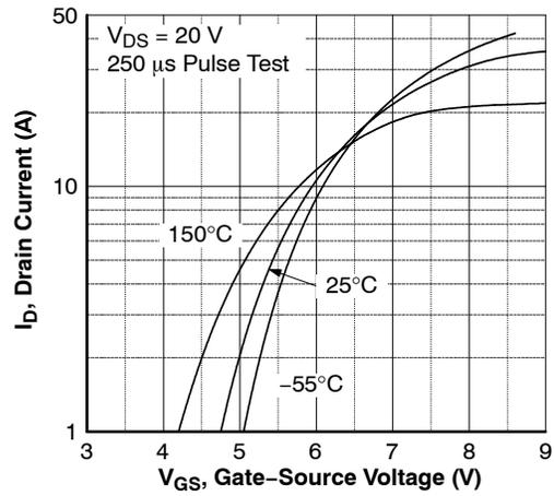
Figure 2. Transfer Characteristics
