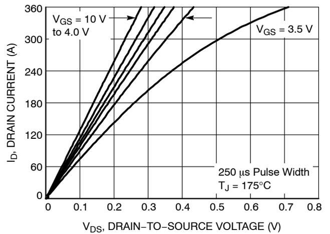
Figure 10. Saturation Characteristics
