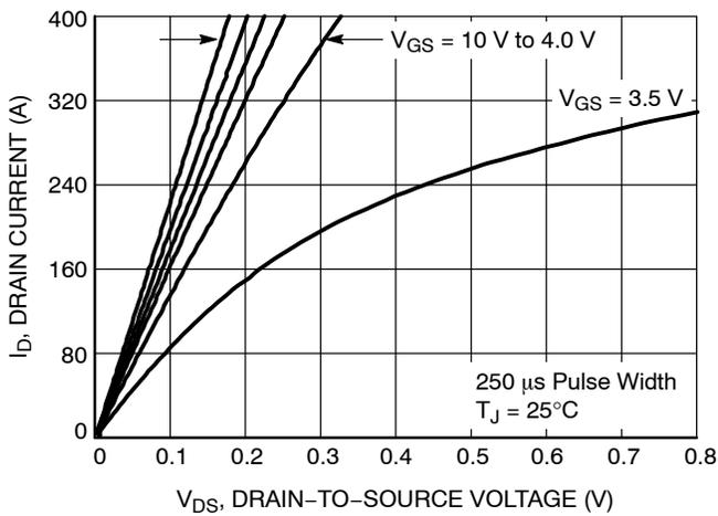
Figure 9. Saturation Characteristics
