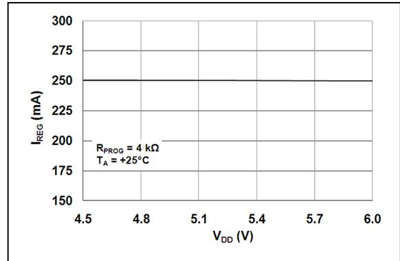
**FIGURE 2-12:** Charge Current ( $I_{OUT}$ ) vs. Supply Voltage ( $V_{DD}$ ), MCP73830.
