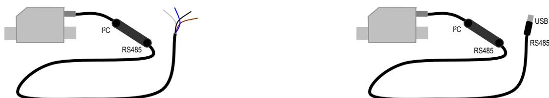
Picture: SCC1 sensor cable connected to sensor with pig tail cable (left) and with USB plug (right). Communication interfaces shown in small print.
