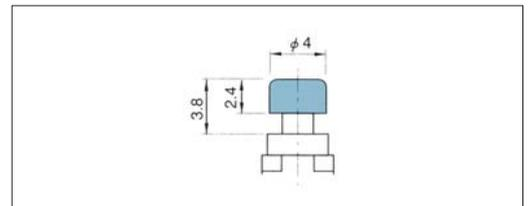
The color cap should be installed after the reflow soldering and washing process.
