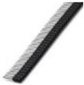
Taped ferrules, 1.5 mm<sup>2</sup>, sleeve length 8 mm, with plastic collar, according to DIN 46228-4, black, for processing with the CRIMPFOX 4 IN 1, 10 strips each with 50 sleeves per strip.
