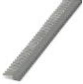
Taped ferrules, 0.75 mm<sup>2</sup>, sleeve length 8 mm, with plastic collar, according to DIN 46228-4, gray, for processing with the CRIMPFOX 4 IN 1, 10 strips each with 50 sleeves per strip.
