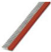
Taped ferrules, 1.0 mm<sup>2</sup>, sleeve length 8 mm, with plastic collar, according to DIN 46228-4, red, for processing with the CRIMPFOX 4 IN 1, 10 strips each with 50 sleeves per strip.
