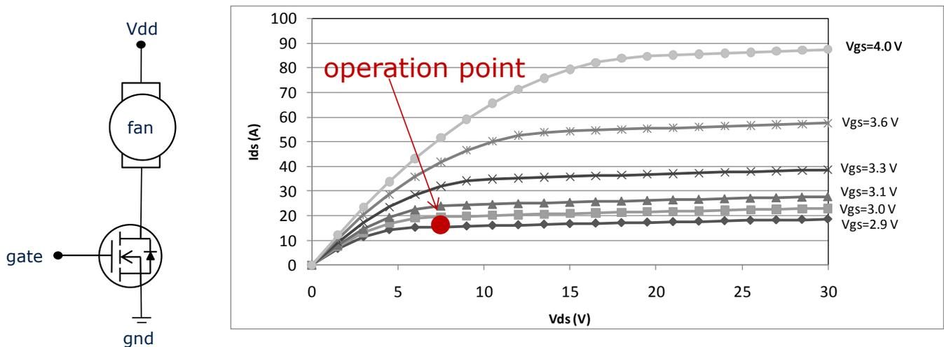
Fig. 2: MOSFET used as constant current source. The current flow through the fan is controlled exclusively by the  $V_{GS}$  voltage at the MOSFET gate. The red point in the output characteristics diagram on the right hand side indicates a potential operation point of the MOSFET in the saturation region.
