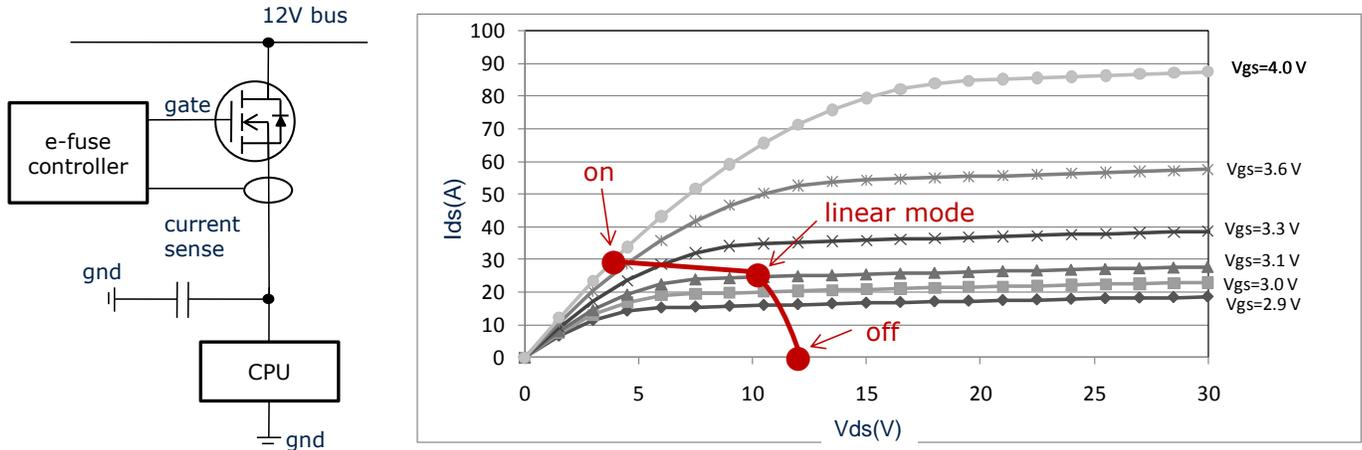
**Fig. 3.** MOSFET used in e-fuse application (left). In e-fuse application (during turn-on) the MOSFET passes the linear mode operation region for a significant period of time. The SOA must be checked to verify the MOSFET can withstand the thermal stress.
