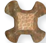
Indenter Crimp Cross-Section Across Axis
