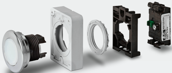
The new M30 mounting system, M30 AFX, adapts automatically to different sheet metal thicknesses, making installation faster and more reliable.
