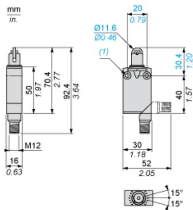
(1) 2 fixing holes Ø 4.2 mm, counterbored Ø 8 mm by 4 mm deep.
