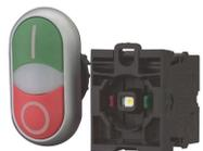
**Double actuator pushbutton, RMQ-Titan, Actuators and indicator lights non-flush, momentary, 1 NC, 1 N/O, White lens, LED element, 85 - 264 V AC, green, red, inscribed, Bezel: titanium**
