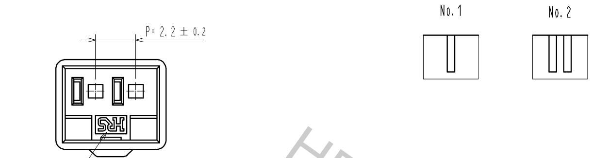
1> FIGURE-1 CONTACT No. MARKING (10:1)
