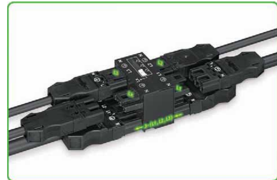
An additional h-distribution connector doubles L1. This results in the following connection options: L1/L1/L2/L2/L3 with jumper in position L2 L1/L1/L2/L3/L3 with jumper in position L3
