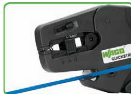
Cutting the conductor.
