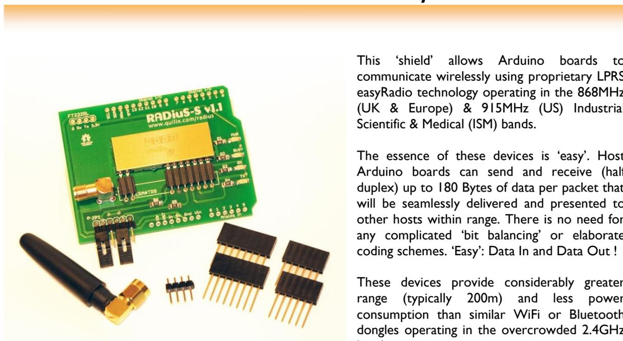
This 'shield' allows Arduino boards to communicate wirelessly using proprietary LPRS easyRadio technology operating in the 868MHz (UK & Europe) & 915MHz (US) Industrial Scientific & Medical (ISM) bands.
