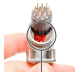
Align Keys to Slots
