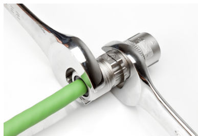
Step 16 - Tighten to 5-7 N/M using 25mm wrench
