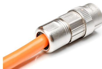
Step 17 - Tighten to 5-7 N/M using 25mm wrench
