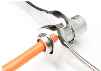
Step 17 - Tighten to 5-7 N/M using 25mm wrench
